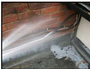
*Simulated rainfall testing of counter flashings*
